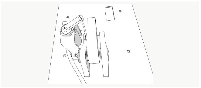
The electromagnet of the safety ratchet is not sufficiently secured and therefore the ratchet does not function smoothly.
